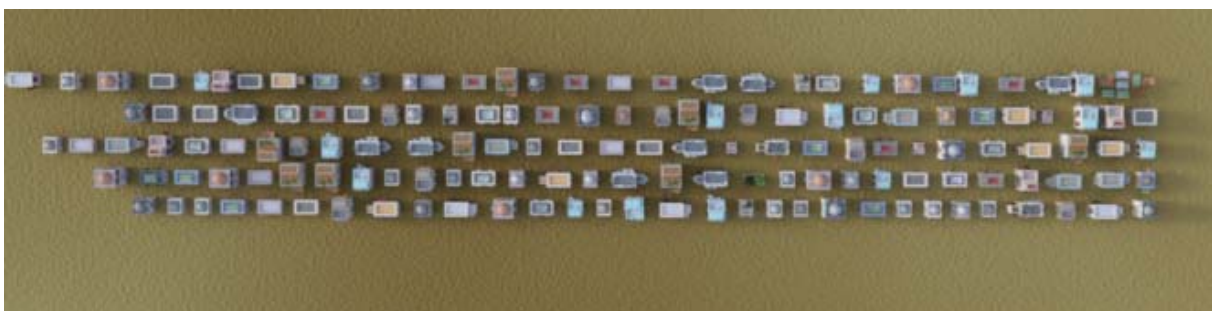
Scene with streets for which the "Percentage of Randomness in Distance Between Elements In The Street" dial has been raised, street after street from 0 (bottom street) to 100% (top street) in 25% steps. The upper street has a less "organized" look than the lower street.
