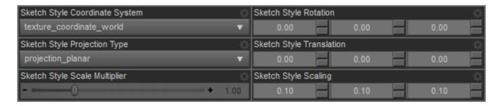
For the sketch styles to apply universally to surfaces without the requirement of specific UV mapped textures it uses some projection mapping which can be altered by the above values. The values here apply to all texture maps in all previously covered settings excluding *Toon Diffuse Color 1*.
