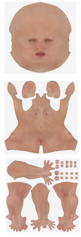
Figure 7: DAZ figure's textures are grouped into 3 UV Maps and divided into SkinFace, SkinTorso and SkinLimbs
